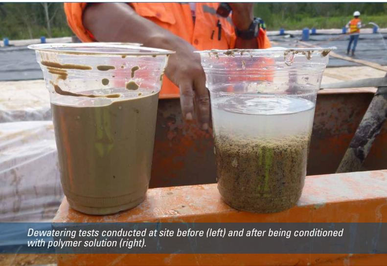
Dewatering tests conducted at site before (left) and after being conditioned with polymer solution (right).
